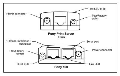
Figure 2-3 Pony Print Server Plus and Pony 100 Switches and LEDs
